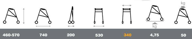
Sizes in mm, weight in kg. Deviations in sizes and weight (15 mm, 1,5 kg and 1,5°) are possible.
