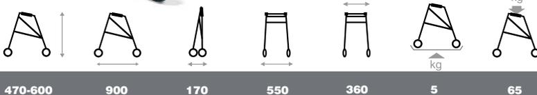
Sizes in mm, weight in kg. Deviations in sizes and weight (15 mm, 1,5 kg and 1,5°) are possible.
