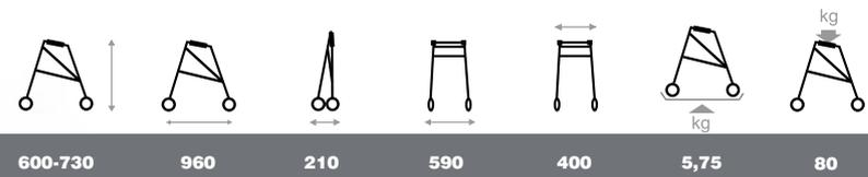
Sizes in mm, weight in kg. Deviations in sizes and weight (15 mm, 1,5 kg and 1,5°) are possible.
